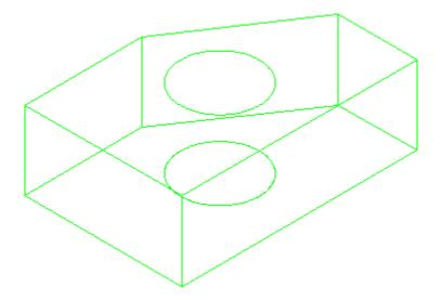
Pick any line and snap to an endpoint grip. Look at the co-ordinate display on the left of your status bar and see if it makes sense to you. Try this at other points. What you have just done is created a simple object in 3D drawing space. It has length, depth and height. Get used to looking at it, and review what you did to create it.
