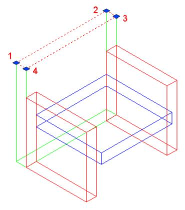
Switch layers and repeat the command to add 3-D faces to the top of the sides and the seat. 3D faces are great for making odd shapes that include any four lines (or arcs) that are touching).
