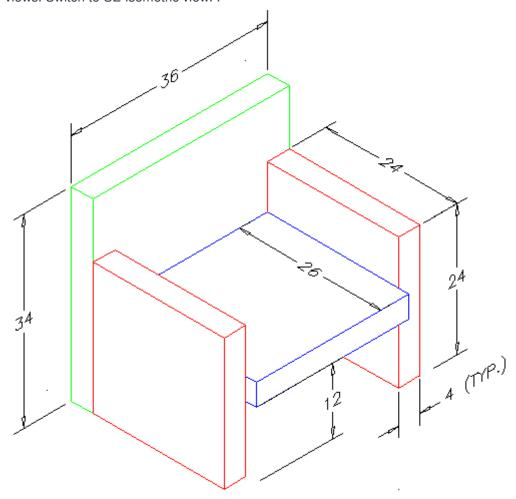
Start with the back. Make rectangle to define the plan view of the back of the chair. Pick or specify the first point (0,0,0) of the rectangle, and for the second point type @4,36. Notice that x, y coordinates were given only. Z distance is 0 by default
