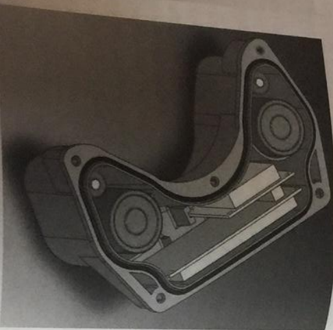
Figure 9.10 Solid models of mated enclosure base, o-ring, batteries, GPS and CPU cards
