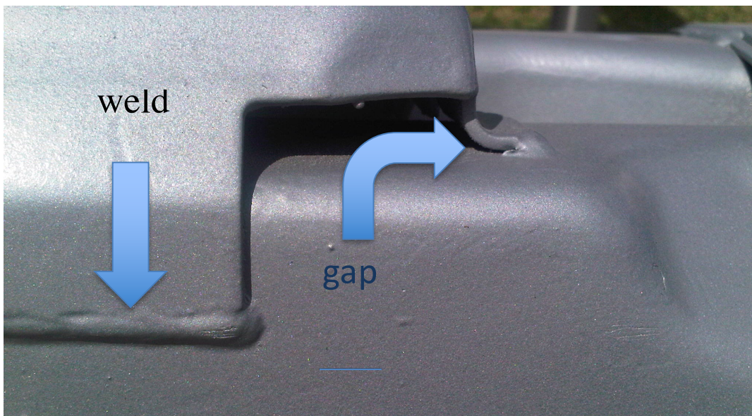
Exhibit 7 Close Up of Structure and Gap After Welding
