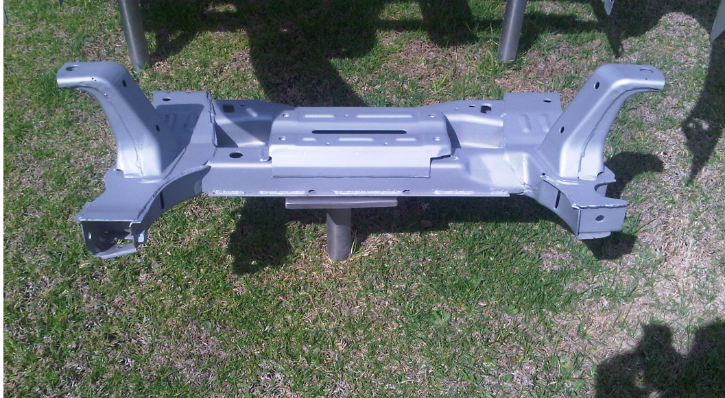
Exhibit 7 Close Up of Structure and Gap After Welding
