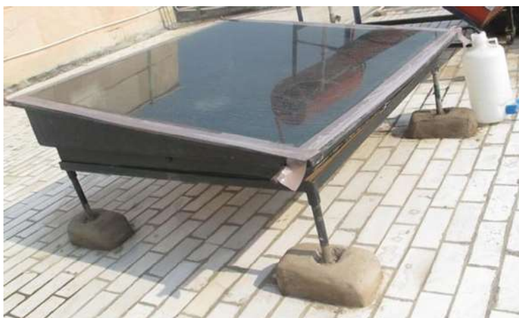
Fig. 3 Single basin-type solar still with distillate collector
