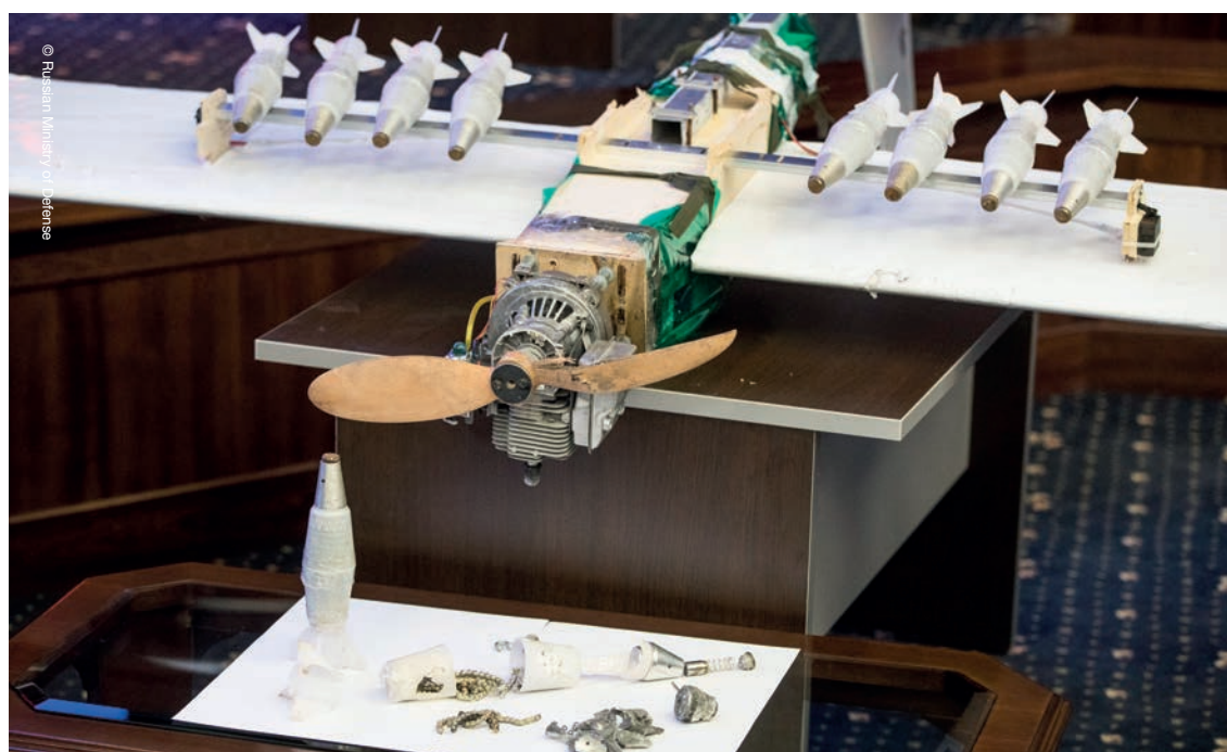
Presentation of DIY build drones used by Syrian armed group for attack on Russian Air Force stationed at Latakia Air Base, Syria, 2018.
