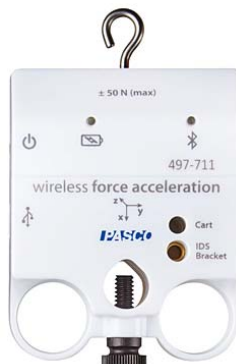
Figure 1. Photograph of the PASCO Force/Acceleration Sensor used during testing.
