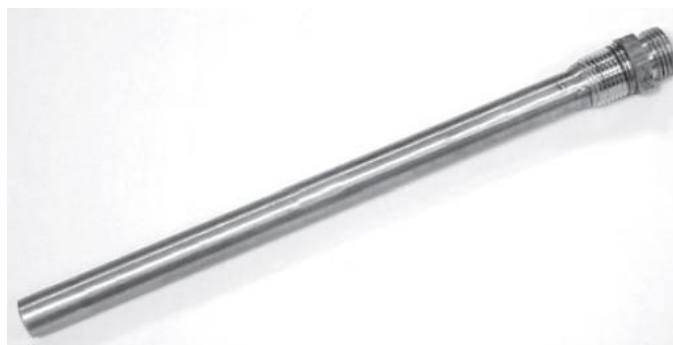
Figure 9. The thermowell or 'Pocket' instrument (TecQuipment Ltd., 2009).
