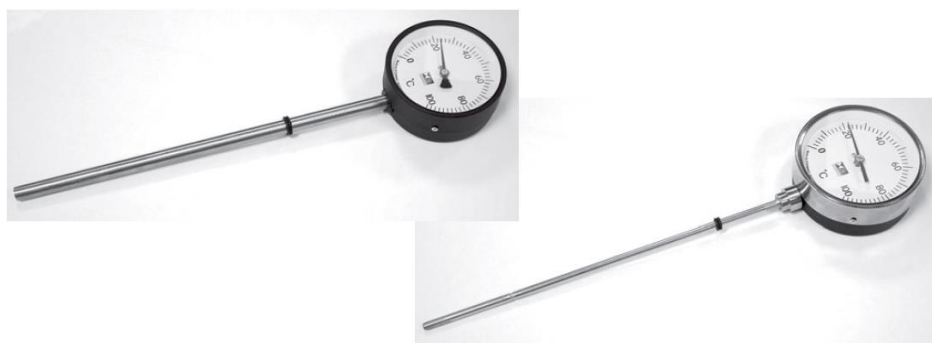
Figure 3. The gas (vapour) and bi-metal thermometers (adapted from TecQuipment Ltd., 2009).
