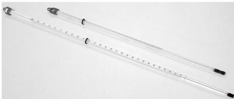
Figure 2. The liquid filled glass thermometers (adapted from TecQuipment Ltd., 2009).
