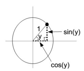
If you imagined this circle to be an electrical generator, spinning anti-clockwise with the dot starting at 3 o' clock, then measurement of the height of the dot versus time would trace out a very familiar sine wave. The mains electricity supply has a sinusoidal nature and this is produced by a circular generator at the power station. For this reason we can say that *trigonometric functions such as sin, cos and tan are CIRCULAR functions*.
