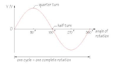
If we say  $\sin(90^\circ)=1$  then what this means, in relation to the sine wave above, is that the sine function reaches an amplitude of 1 at  $90^\circ$ . This is reading the function from the bottom up and then left. What if we were to read the function from the left first of all and then across and to the bottom? This could be expressed mathematically as...
