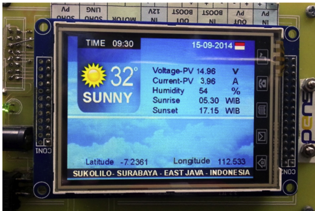
Fig. 4. Prototype of PV monitoring system.
