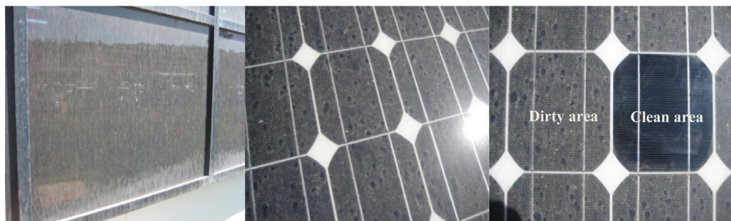
Fig. 3. Pictures of accumulation of Dust layer on PV modules in North Algeria (Tipaza region) on 29th May 2016 confirming SKIRON online results data maps.
