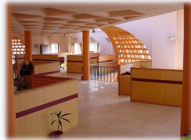
SOLAR SHELL OR LIGHT VAULT
