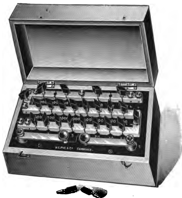
Fig. 61. Wheatstone Bridge Resistance Box.
