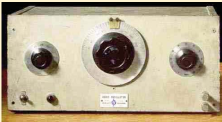
Hewlett-Packard's first product: an audio oscillator
