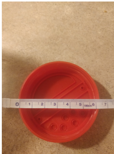
Figure A.7: Measuring the diameter of the boat. We find its diameter is 6.1 cm.
