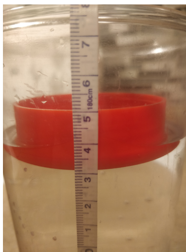
Figure A.4: The boat without mass is approached to the same side as the ruler to log its initial depth. We measure it to be 3.1 cm.
