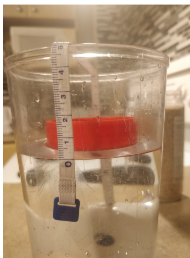
Figure A.2: The setup of this experiment. A transparent cup is filled with water and a plastic cap is floating at the top. A ruler is used to indicate the water level, which sits initially at 0 cm.
