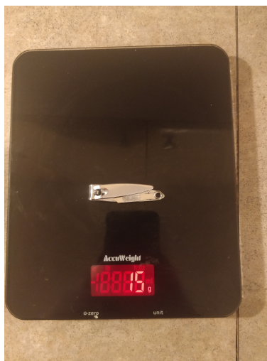
Figure A.1: The mass of the clipper which will be measured using Archimedes' principle. Its mass is 15g according to a kitchen scale.
