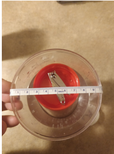
Figure A.6: Measuring the diameter of the cup. We find its diameter is 9.5 cm.
