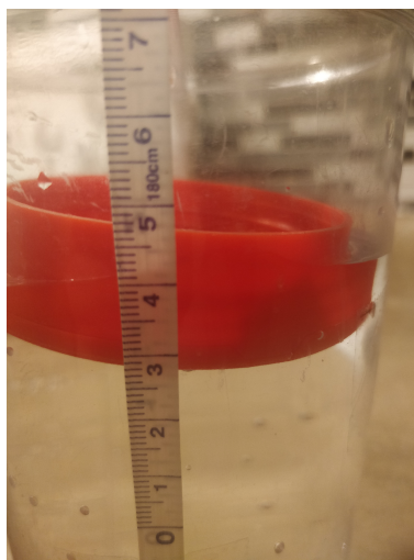
Figure A.5: After the mass is added to the boat, we log the new depth which falls to about 2.85 cm.
