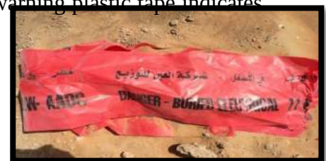
Fig 2.1.10 Warning plastic tap
