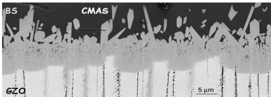
50 Dissolution of gadolinium zirconate ( \text{Gd}_2\text{Zr}_2\text{O}_7 ) into the CMAS melt results creates a dense, impervious layer/zone that prevents or significantly slows down further penetration and reaction 178
