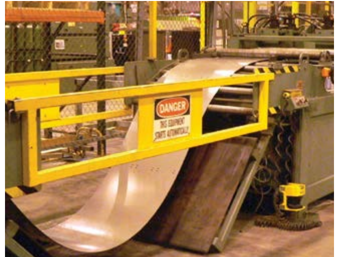
S3000 Safety Laser Scanner Mounted on a Coil Processing Line
