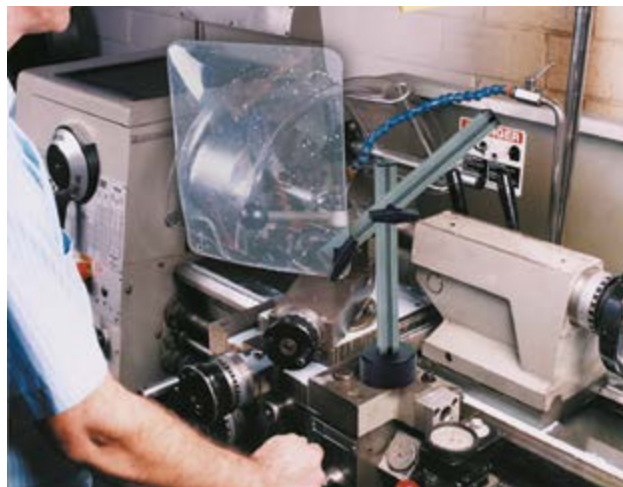
Magnetic-base concave shield shown on a lathe
