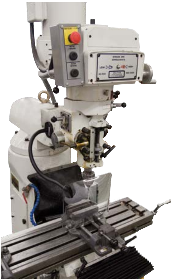
Flexible spring-steel arm shield on milling machine.
