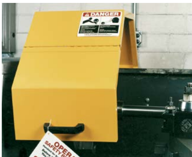
The hinged portion can swing up for workpiece changes.
