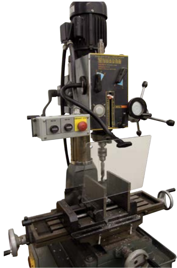
Flexible spring-steel arm shield on milling machine.
