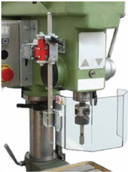
Electrically interlocked shield for small to medium size drill presses.
