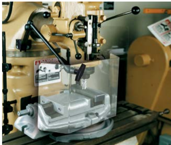
Universal ball & socket shield on a milling machine.
