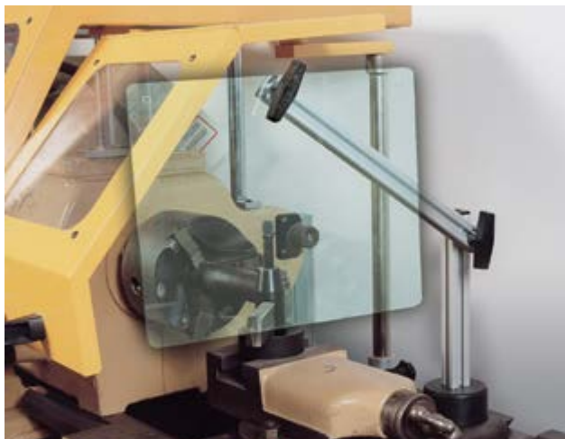
Magnetic-base flat shield shown on a lathe
