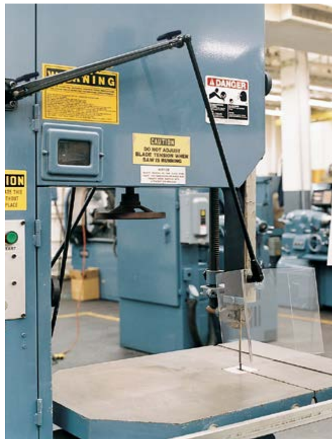
Universal ball & socket shield shown on a band saw.
