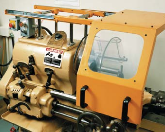
Shield slid into position. Machine is ready for machining workpiece.
