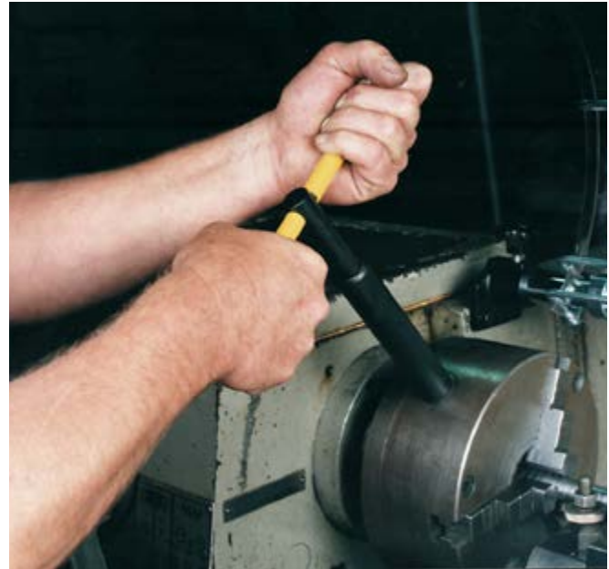
Adjusting the chuck using a spring-loaded chuck wrench.
