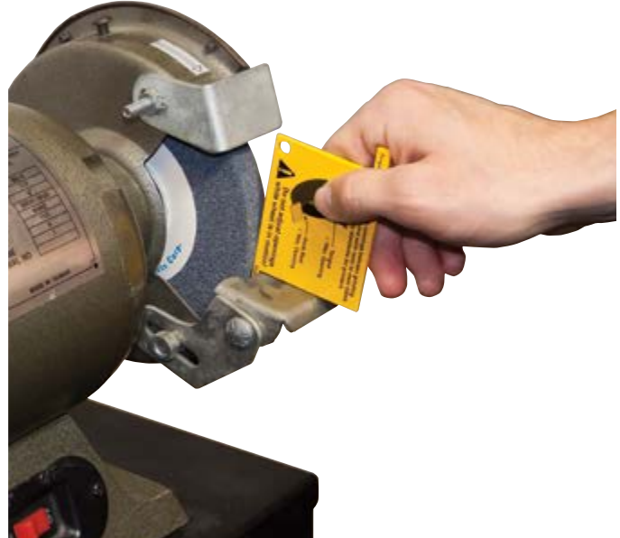
Checking work rest opening.
