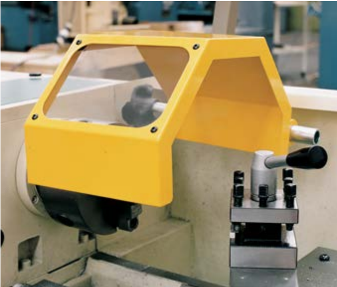
Shield in position. Machine is ready for machining workpiece.
