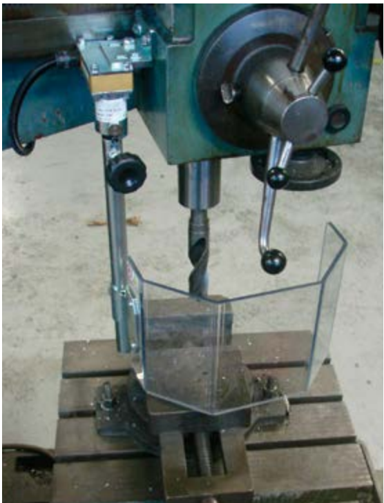
Electrically interlocked shield for larger drill presses and radial drill presses.
