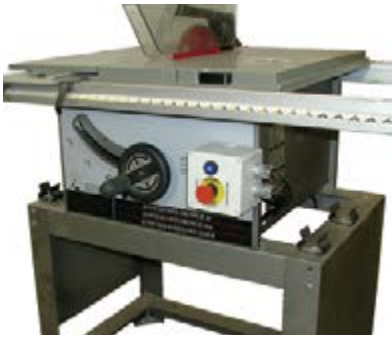
SAFS-300 Sensing-Saf-Start® package on a table saw.
