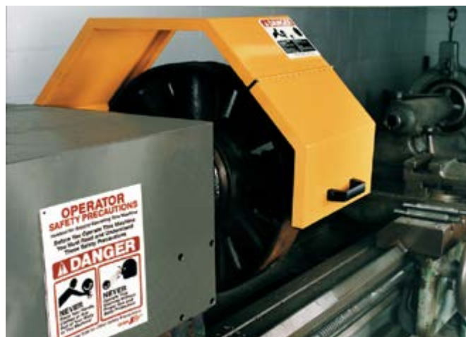
The hinged portion can swing up for workpiece changes.
